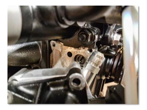
Fit the 3 X bolts and tighten to 10-14NM.
