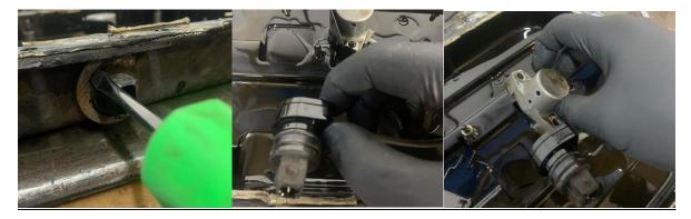
11. The underneath of the engine must be cleaned and removed of all silicone residue prior to fitting the RRP Sump.
