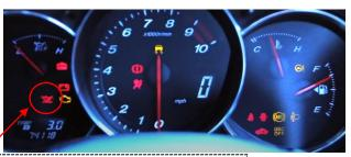
Push Level switch down and observe Low light operation on the Instrument cluster.
